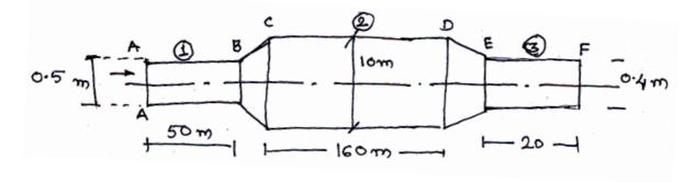
For the above duct system inlet velocity of air at A-A is 540 m/min. Loss in  $(B-C) = \frac{1}{2} \times \text{velocity}$  pressure in (A-B), Loss in  $(D-E) \frac{1}{5} \times \text{Velocity}$  pressure in (E-F) using friction loss equation  $P_f = \frac{0.263 \text{ C}^{1.85}}{D^{1.27}}$ , where
